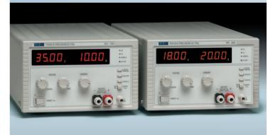
Specifications: Line & load regulation <0.01%. Output noise <1mV rms. Meter accuracies 0.2%  $\pm 1$ digit - voltage, 0.5%  $\pm 1$ digit - current.
