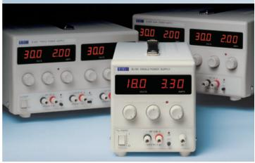
Specifications for Main Outputs: Line & load regulation <0.01%. Output noise <1mV rms. Meter accuracies 0.3% ±1digit - voltage, 0.6% ±1digit - current.
