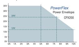
The CPX200 can provide up to 350 watts (175W per channel). As the set voltage is reduced below 35V, the maximum output current is increases up to a maximum of 10A.
